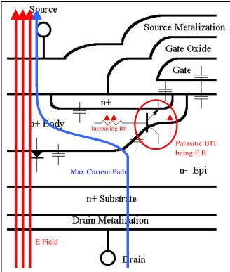
Figure 8: Power MOSFET Cross Section Under Avalanche
