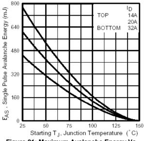
Figure 21: Maximum Avalanche Energy Vs. Temperature For Various Drain Currents
