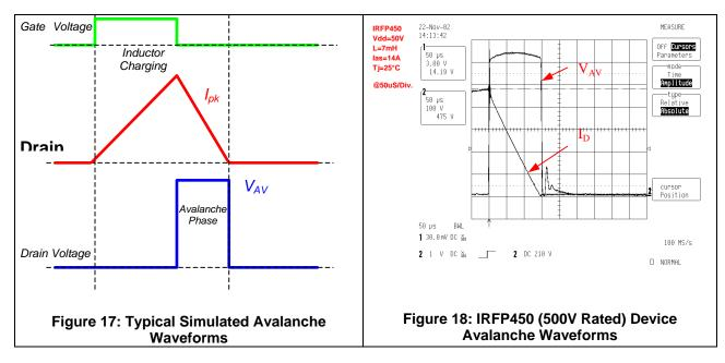
Note that the peak avalanche voltage  $V_{AV}$  can be approximated as 1.3 times the device rating, or 650V. Further note that  $V_{(BR)DSS}$  and  $V_{AV}$  are used interchangeably in this text.
