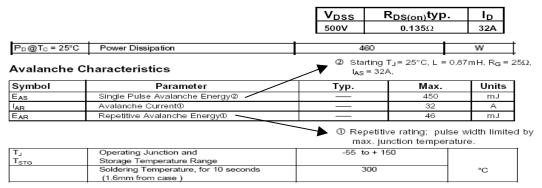
Figure 19: IRFP32N50K Data Sheet Excerptions
