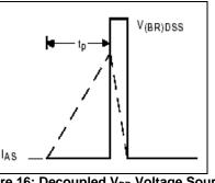
Figure 16: Decoupled V<sub>DD</sub> Voltage Source Test Circuit Waveforms
