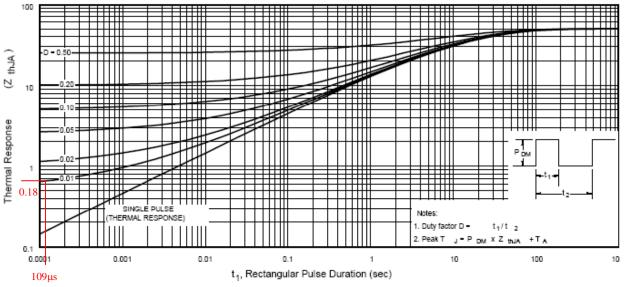
Figure 25: IRF7484 Typical Effective Transient Thermal Impedance, Junction-to-Ambient
