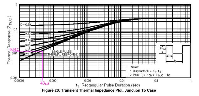
The temperature increase due to avalanche and the final junction temperature can therefore be calculated using Equation 4
