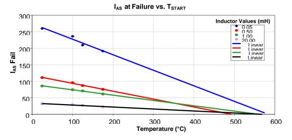
Figure 12: I<sub>AS</sub> at Failure Vs. Test Temperature
