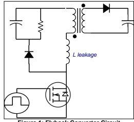
During MOSFET operation of the Flyback Converter, energy is stored in the leakage inductor. If the inductor is not properly clamped, during MOSFET turnoff the leakage inductance discharges through the primary switch and may cause avalanche operation as shown in the  $V_{DS}$ ,  $I_D$ , and  $V_{GS}$  versus time waveforms in Figures 2 and 3.
