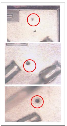
Figure 10: Power MOSFET Random Device Failure Spots
