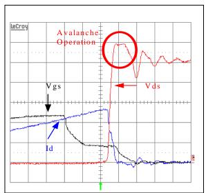
Figure 3: Flyback Converter Switch Under Avalanche Waveform (Detail)
