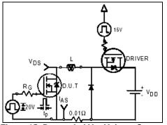
Figure 15: Decoupled V<sub>DD</sub> Voltage Source Test Circuit Model
