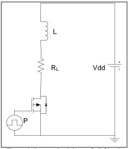
Figure 4: Automotive Injector Coil Circuit
