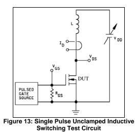
From the Figure 13 schematic we can calculate the single pulse avalanche energy  $(E_{AS})$  as:
