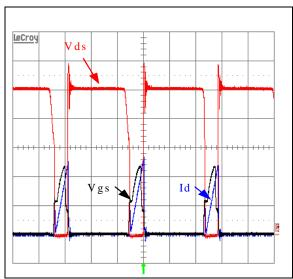
Figure 2: Flyback Converter Switch Under Avalanche Waveform
