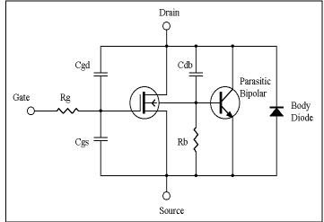
Figure 7: Power MOSFET Circuit Model
