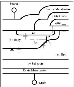
Figure 6: Power MOSFET Cross Section
