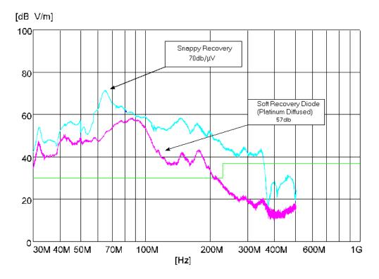
The softness is related to the quantity of charges left in the n- region after the full spread of the depletion zone in blocking mode. To sustain the demand of the current of the external stray inductance, allowing the current to return to zero in a smoother way, the charge left in the n- region must not be too low.
