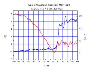
With this type of performance, the maximum allowable switching frequency for this Ultrafast diode family would be up to 500-750kHz. This assumption is verified by the diode loss calculation used for the IR MUR1620 operating in a typical output rectification in a forward converter. Let's assume a current load of 8A @ 60% duty cycle, with a switching di/dt of 200A/µs and an over-voltage of 100V with the diode operating at the maximum junction temperature.
